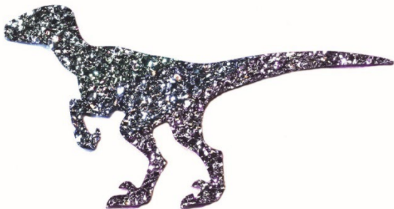
Image: Wire cut by wire erosion process
